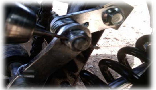
STEP 3: Insert Cotter-pin
