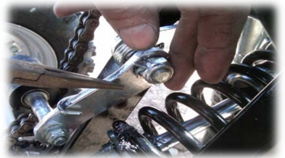
STEP 4: Fold legs of pin over sides of nut
