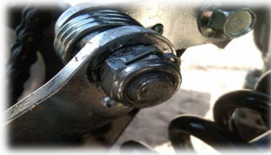
STEP 5: Fold legs of pin over sides of nut
