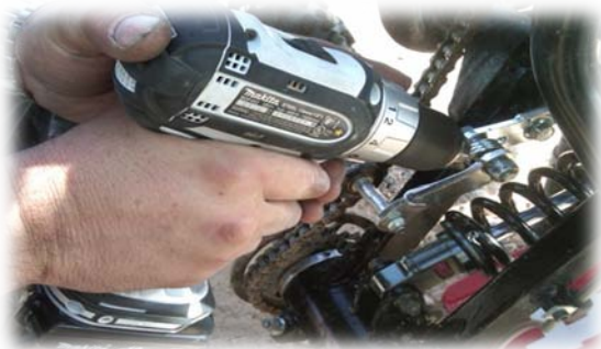
STEP 1: Drill the 17mm Nut using a Cobalt drill-bit
